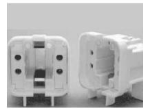
Specifications for Part Number (FL423V-Q1):• Quick connect pushin wire terminals for 18 AWG Solid or Twist & Tin stripped 7/16 in.• Rated 75W, 600V. • Each wiring ports excepts 2 wires for easy harness wiring. • Two hole screw mount on base plate.
