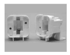
Specifications for Part Number (FL423V-D3):• Quick connect push-in wire terminals for 18 AWG Solid or Twist & Tin stripped 7/16 in.• Rated 75W, 600V. • Two wire ports per terminal to speed harness wiring. • Two hole screw mount on base plate.
