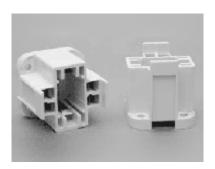
Specifications for Part Number (cf13G24-Q1):• Quick connect pushin wire terminals for 18 AWG Solid or Twist & Tin stripped 7/16 in.• Rated 75W, 600V. • Each wiring ports excepts 2 wires for easy harness wiring. • Four holes on base
