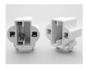
Specifications for Part Number (CF13-HSI): Quick connect push-in wire terminals for 18 AWG Solid or Twist & Tin, stripped 7½16 in. • Snap-in mount into 0.025-0.040 in. (0.6 - 1 mm) panel thickness • Each wiring port accepts 2 wires for easy harness wiring, no extra jumpers or wire nuts to assemble • Rated 75W, 600V.
