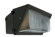
BOROSILICATE MOLDED GLASS, DIE CAST HOUSING, GASKET, CHROMATE CONVERSION COATING, TEXTURED BRONZE FINISH, DUROID BARRIER, ALUMINUM REFLECTOR, PORCELAIN MOGUL SOCKET & BRACKET, REUSABLE STYROFOAM & INNER CARTON
