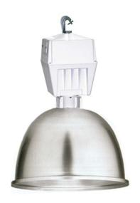
DIE CAST HOUSING WITH ACCESS FOR WIRING, ACCOMODATES 1000 WATT METAL HALIDE OR HIGH PRESSURE SODIUM BALLASTS, PORCELAIN MOGUL BASE SOCKET, 1" THREADED HOLE ON TOP FOR HOOK OR PIPE, INCLUDES MALLEABLE HOOK WITH SCREW AND DELUXE ACCESSORY BRACKET FOR MOUNTING REFLECTORS/REFRACTORS. WHITE POWDERCOAT FINISH.
